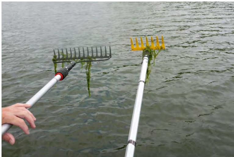
Figure 4. Rake samplers: the rakehead on the left has 14 tines and 33 cm wide and was used for density determinations. The rakehead on the right has 7 tines and is 15 cm wide and was used for biomass sampling.
